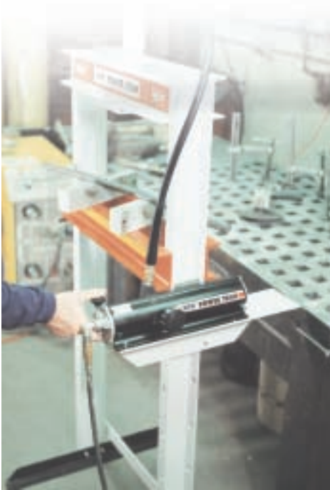
PA9H Hand Control Pump as used in a straightening press.
